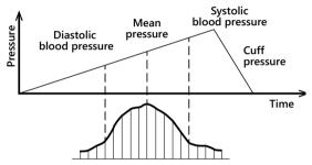
the pressure sensor collects the pressure amplitude changes in the cuff, converts it into a digital signal and sends it to the CPU. The embedded software is used to analyze and identify the corresponding pressure points in the process of arterial blood flow obstruction to determine the diastolic, systolic and mean blood pressure of the human body.
